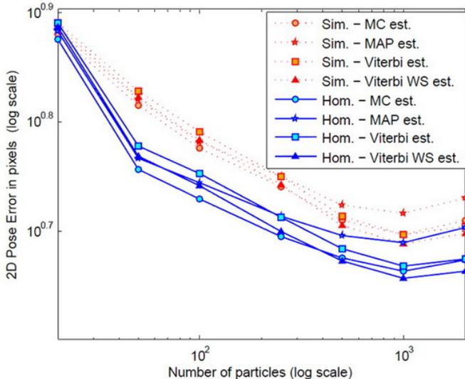
Fig. 11. Average 2D pose error varying the state estimator: performance over 20 runs of the tracking algorithm on the 11 tracks for homographic and similarity alignments. We present the RMS 2D pose error when estimating the state at each time step using the Monte Carlo approximation (MC), the MAP criteria, Viterbi path finding algorithm (Viterbi) and the weighted sum around the Viterbi estimate (Viterbi WS).
