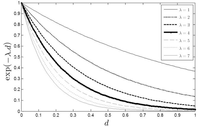
Fig. 5. Likelihood function as a Laplacian distribution  $\exp(-\lambda d)$  over the distance  $d \in [0, 1]$  for several values of the parameter  $\lambda$ . In this work, we consider an acceptable Likelihood function is obtained with  $\lambda = 4$ .
