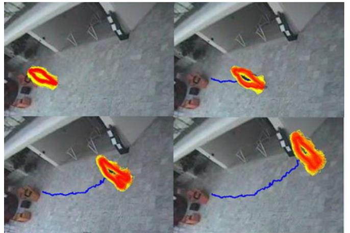
Fig. 8. Visualization of the likelihood for the entire sample set in several frames of the Walk2 sequence. For each frame, we plot the set of sampled and aligned shapes: darker colors indicate a higher likelihood.
