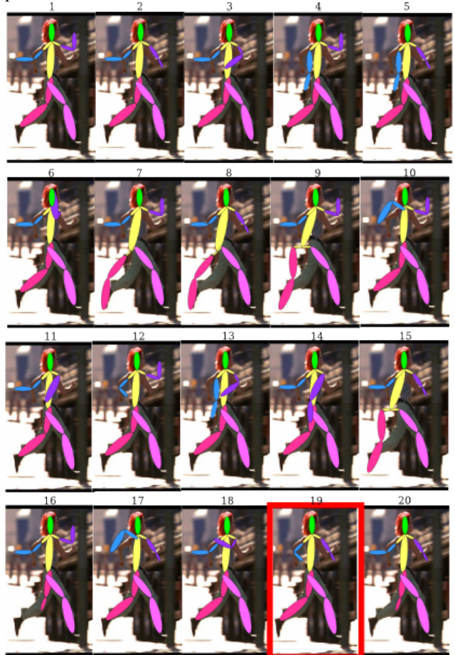
Figure 7. We show the 20-best configurations returned by our N-best algorithm for a frame in the Lola video. Note that each configuration contains at least one part that does not overlap any other configuration. Since there exists arm-like clutter at the top of the image, many of the top-scoring hypotheses consider various arm positions. Note that many of these configurations share the same root; hence they would not returned from typical NMS-based algorithms for generating multiple detections in an image. We show final configuration selected by the DP tracker in red , which was the 19-th returned pose.
